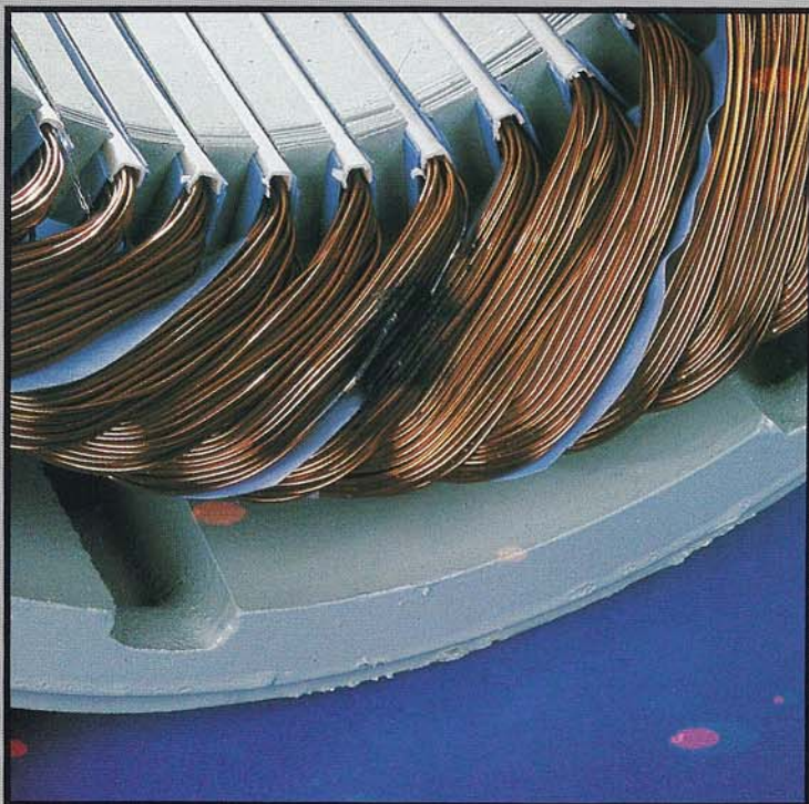
3 Winding Shorted Phase-To-Phase
