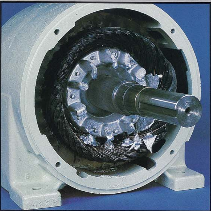
11 Damage Caused by Locked Rotor
