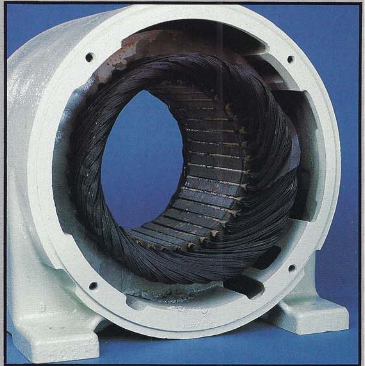
10 Winding Damaged Due to Overload
