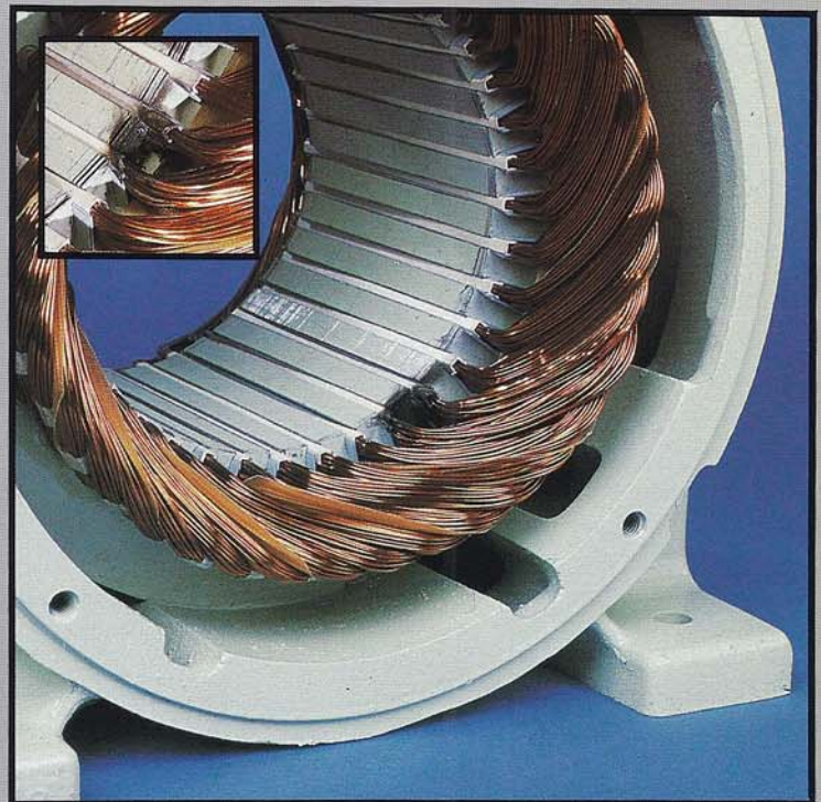
6 Winding Grounded at Edge of Slot
