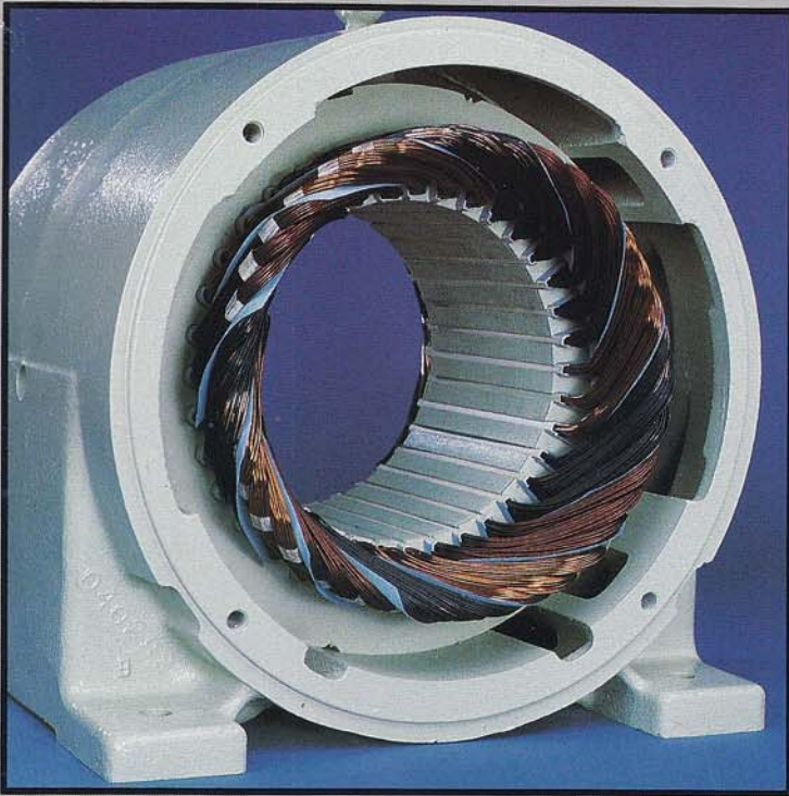
9 Phase Damage Due to Unbalanced Voltage
