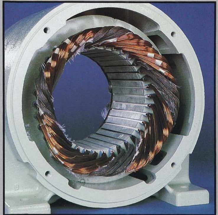
2 Winding Single-Phased ( \Delta - Connected)
