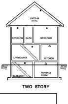
Key • Smoke Alarm ∆ Smoke Alarm with False Alarm Control™
