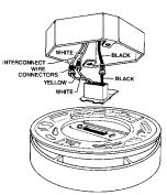
10. Position smoke alarm to mounting plate and turn clockwise to lock into place. For tamper-resist, use long-nosed pliers to remove thin plastic from notch on smoke alarm edge. Insert pin into notch on edge of smoke alarm after smoke alarm is positioned properly in base.
